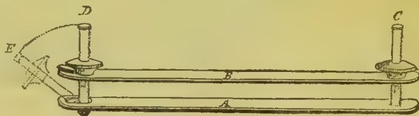
FIG. 71.—Clamp for isolating a portion of the intestine. (Colin.) A, lower plate; B, upper plate; C, fixed screw; D, movable screw in place; E, screw turned so as to allow the clamp to be passed around the intestine.
